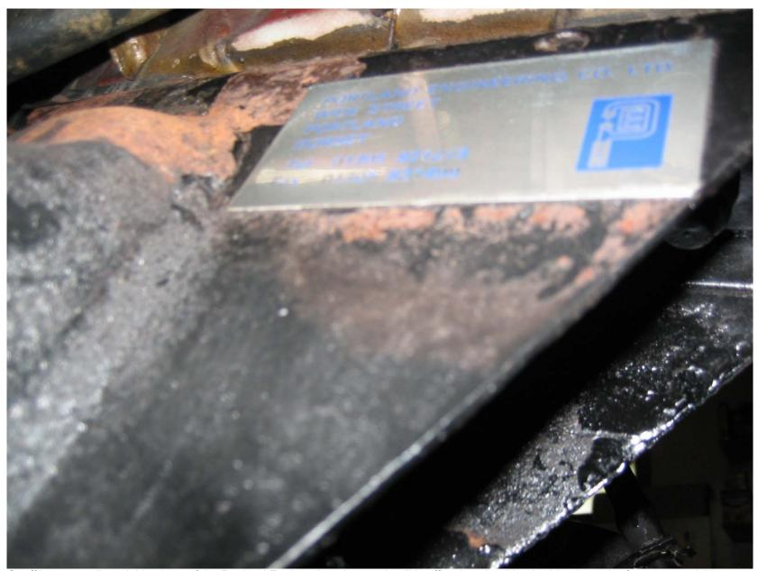
Geoff Lane contributed this photo of the Portland Engineering plate saying "It's affixed on the driver's side above the front upper wishbone mounting point. The dimensions are: Length 9cm, Width 4.5cm." – see the V8 Bulletin Board thread below.
