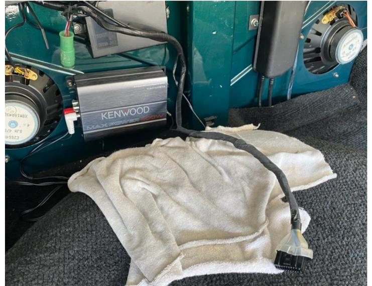
Image 4: Boot wire harness now complete with loom tape applied
