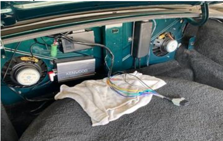
Image 2: Detailing adjustment to vehicle loom and new Kenwood amplifier plug now incorporated into harness
