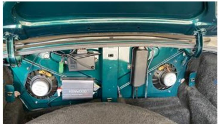
Image 5: Kenwood amp fitted in place of original amplifier using one speaker fixing and one original amp fixing, loom/harness now tucked behind central pillar, Red & White RCA plugs coming up from the carpet to connect to the amp via the small hole that exists within the rear panel towards the bottom left.
