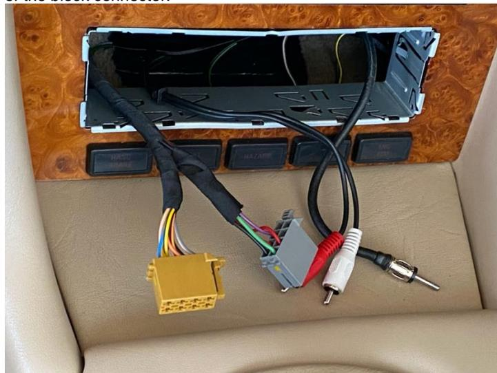
*Image 1: Standard IOS plugs Grey and Tan, with additional amp trigger wire fitted to grey plug next to green power supply, additional Red and White RCA (Radio Corporation of America plugs) that will connect directly to the amp*
