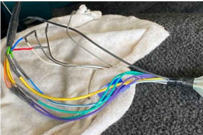
Image 3: You can see here I have removed the original vehicle plugs for the speaker connections and amp connections and soldered the Kenwood supplied loom to the two speaker outputs (orange & yellow wires), the fused power which is already in the boot (dark green) the amp trigger which is coming from the radio ISO plug (light green) as detailed in image 1 and finally the earth black wire, to the original harness that resides in the boot
