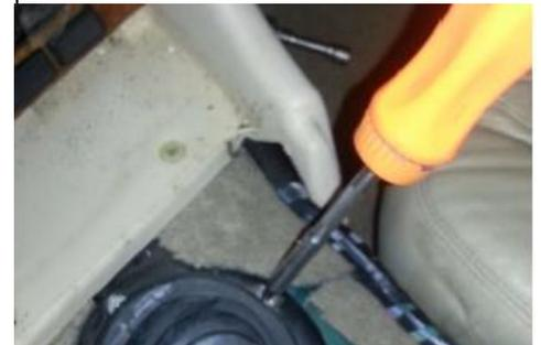
If your hands are large, like mine, then widening the hole exposed by the forward access panel can be achieved by two sideways saw cuts to the right and bending up a flap of the transmission tunnel metal. The gear lever extension housing mounting bolts can be removed with various spanners sockets/extensions, etc.
