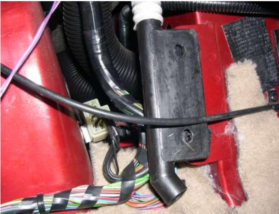
tunnel kick-panel (the one with the interior light) which not only reduces the effective hose diameter but additionally forces the air to deviate considerably. This moulding is a push fit into the light-grey cross-facia hose and also onto its mountings - the backs of the pads that carry the Velcro-like fasteners for the forward end of the kick-panel.
