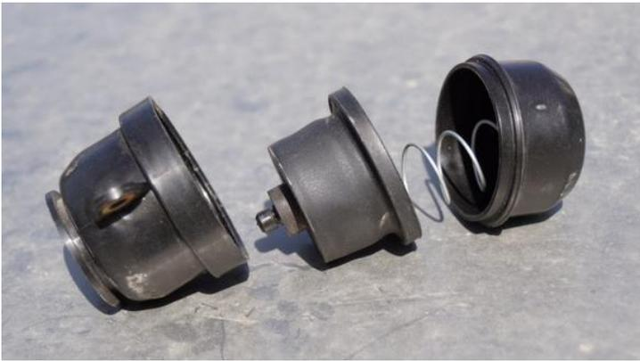
**Dismantled plastic vacuum actuator.** The outer ridge on the smaller part on the right just snap-fits into the inner groove on the larger part on the left that has the attachment lugs moulded on it, so it's just brute force to separate them! (Photos: Derek Squires)
