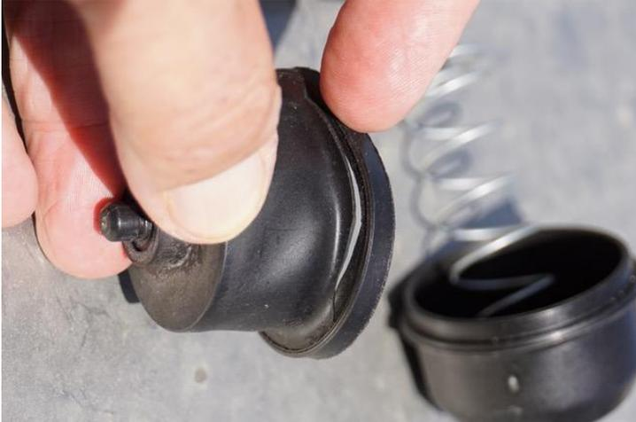
You can see here the **rubber diaphragm splits along the edge**. Using Superglue would only be a temporary fix.
