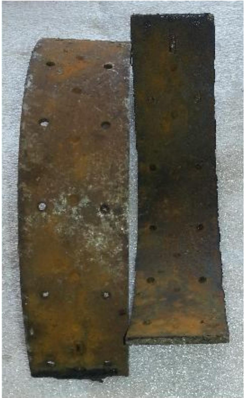
**Brake linings in trouble** – they are suffering from a failure of the bond between the lining and the metal shoe. This dangerous condition is not revealed by the brake test on the rollers which is part of the annual MOT test. It's essential the annual service, whether carried out by the owner or by a service garage, includes the removal of the wheels and an inspection of the brake linings and brake cylinders.
