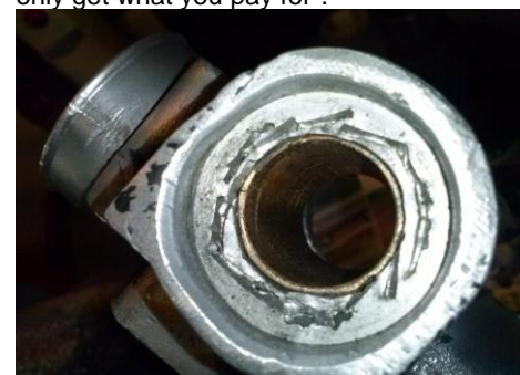
Poor quality work with the pinion there and seal inside.
