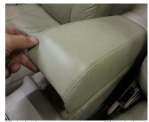
Lift the **leather arm rest** and release it from the four black self-gripping pads underneath (see two of those pads below).
