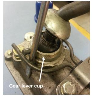
Take a flat bladed screwdriver or pry bar and lever the **bias spring arms** from over the gear lever cross pins (see left) on both sides so each spring arm is then below the cross pins (see below). The bias spring ensures the resting place for the gear lever when out of gear is in line with gears 3 and 4. The cross pins are part of the gear lever ball.
