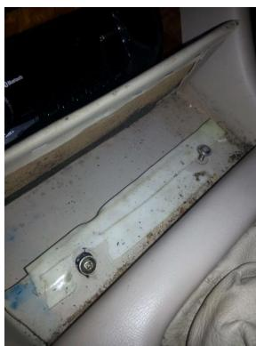
Next you need to remove the **trim pad under the radio** and take out the last two screws.
