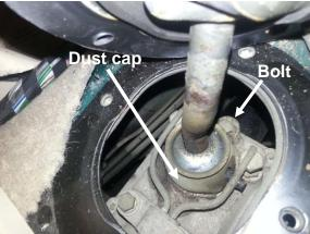
Now remove the bolt holding down the **bracket on the side of the dust cover cap** – you may find at this stage that the bracket has broken so you will either need to replace it or repair it. You can see above that the access to carry out this service work is very restricted and tight.
