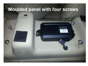
Pull the leather arm rest clear of the four pads which reveals the black volumetric alarm unit mounted on a cream coloured **moulded panel**. Disconnect the plug from the volumetric unit and then loosen the four cross head screws which secure the moulded panel.
