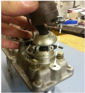
Pull the dust cap up and tape it up out of the way.
