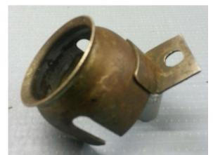
The single bracket on the side of the dust cap is bolted to the body of the gearbox remote control housing. With only one fixing point, movements of the gear lever as gears are selected cause the cap to flex and over time the bracket or cap can break.
