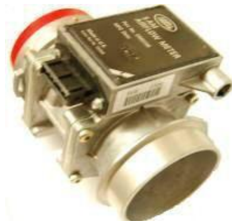
Mass airflow meter was part number ERR 5198 and is now ESR 1057 for a new one
