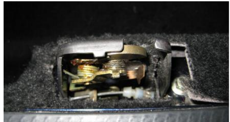
Boot lid is closed - Photo 10 shows the position when the lid is closed – the tab is not in contact with the spindle, the circuit is broken and the interior light goes off.
