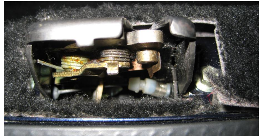
Boot lid is open - Photo 9 shows the position when the boot lid is open - you can see the tab in contact with the spindle, and therefore the interior light is on.
