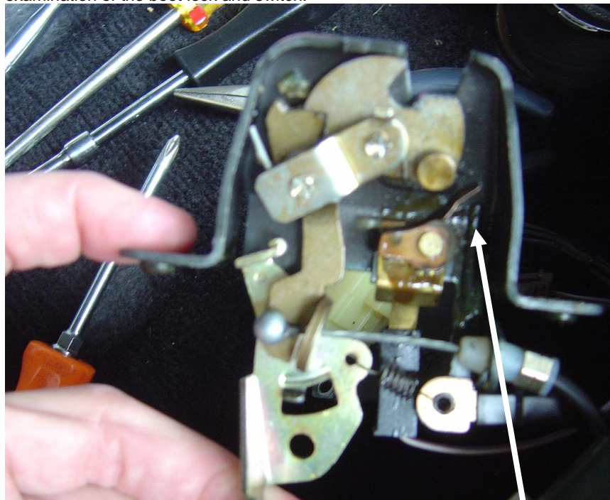
Metal tab shown was bent out of position causing the faulty boot light. (Simon Austin)
