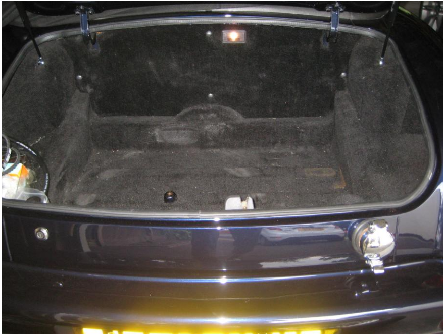
Boot lid is open - Photo 9 shows the position when the boot lid is open - you can see the tab in contact with the spindle, and therefore the interior light is on.
