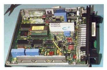
Ensure that the correct Tune Resistor is fitted to the vehicle. This will be marked on the ECU and EPROM chip labels, and varies according to application.
