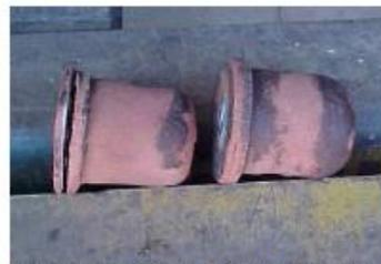
The rubber bump stops on my RV8 had started to crumble and disintegrate (see pictures alongside) and were in need of replacement as the bump stops are an important part of the suspension. After purchasing a new set of upgraded Polyurethane bump stops from Clive Wheatley, I could find no reference for the removal and replacement procedure, hence this note.
