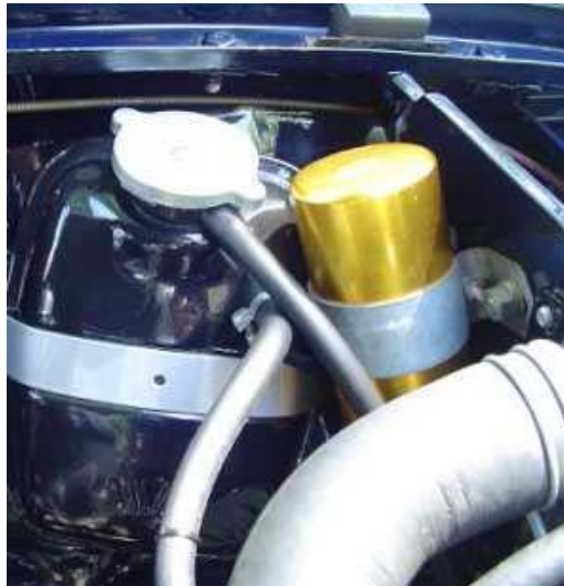
New coil fitted on the nearside radiator panel in the engine bay next to the radiator expansion tank.
