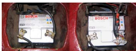
Twin 12V BOSCH 4FN batteries in parallel provide improved starting performance and a near original look. (Photo: Kai Knickmann)
