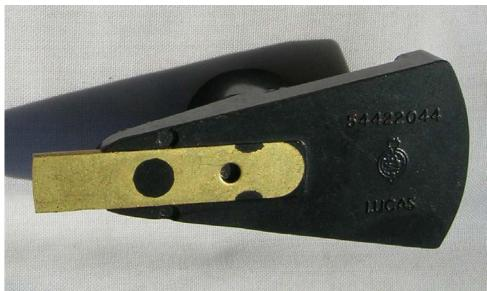
arm, to earth out down the distributor shaft. Result - no sparks at the plugs.
