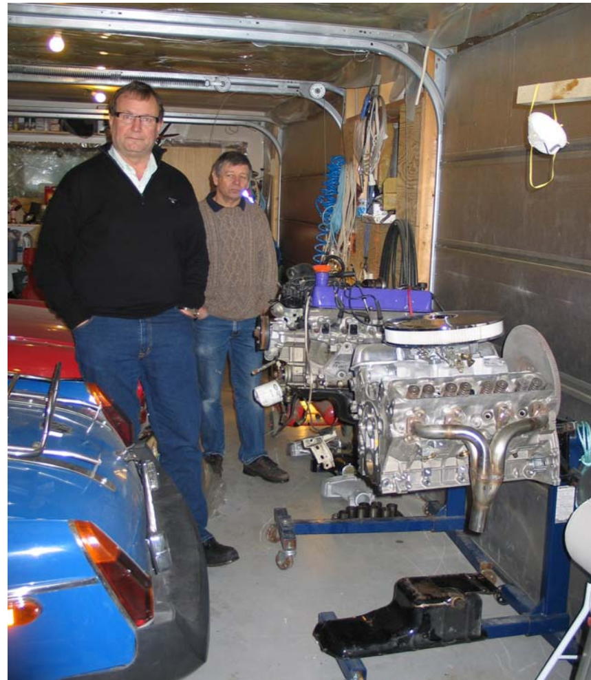
Two V8 engines waiting to be installed in Halvor's MGBs. The Tartan Red '1967 MGBGT will have the 4.6 Rover V8, an LT77 gearbox, an MGC rear axle, Princess 4 pot calipers and Peugeot 604 front brakes. The 1977 NAS spec MGB Roadster in Tahiti Blue will have the TVR 500 engine, Borg Warner T5 gearbox, Hoyle Eng front and rear suspension upgrades and more.
