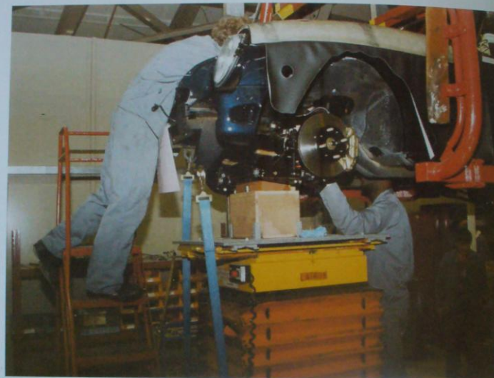
Steve Cook (l) and Noel Johnson (r) work on the Front Cross Member Assembly being secured in position at Station 5 after having been raised into position on Stuff Up Lift Assist (Richard Higgins/BMW Group)
