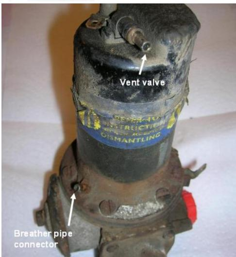
Checking the breather pipes on an SU fuel pump
