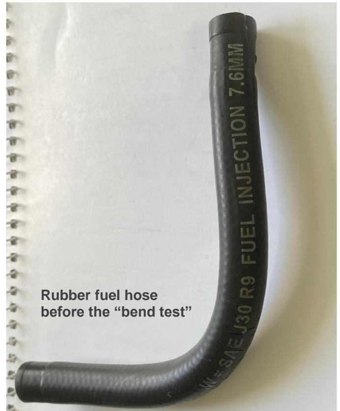
Rubber fuel hose before the “bend test”
