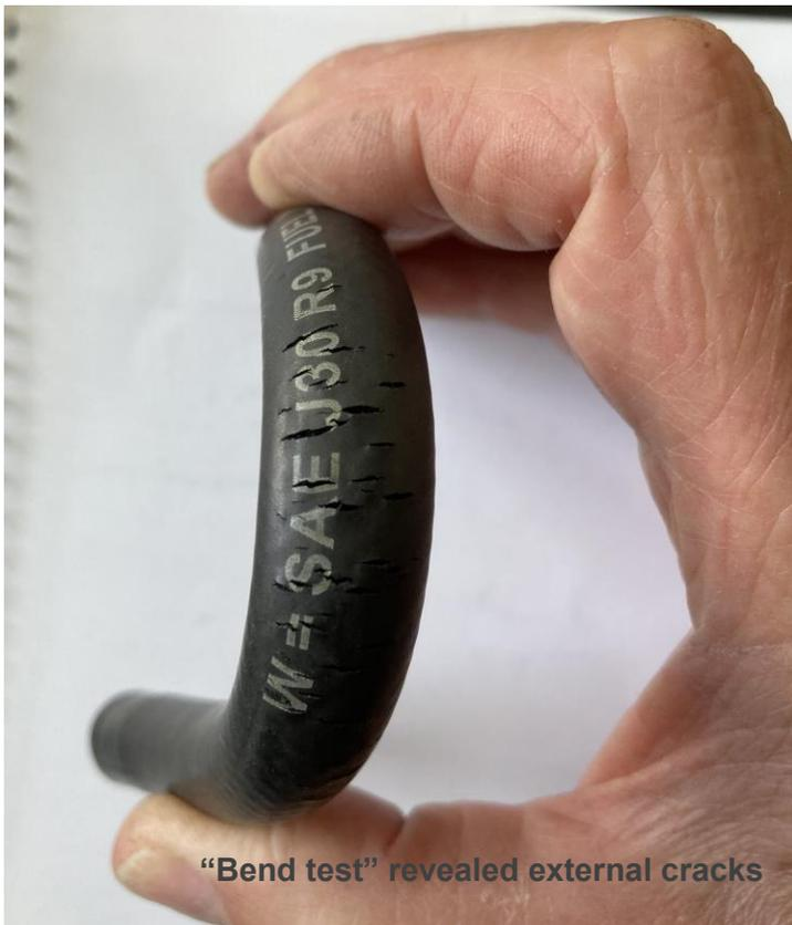
“Bend test” revealed external cracks
