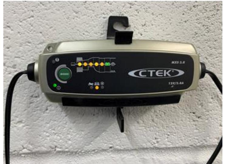
drive the battery terminal voltage up to the charged potential of about 14.6 Volts, and it would then continue to charge at maximum. At this point the charger may overheat if left on continuously. A 12 amp charge rate is quite a heavy current and any doubtful connections might be a source of overheating and possible ignition.
