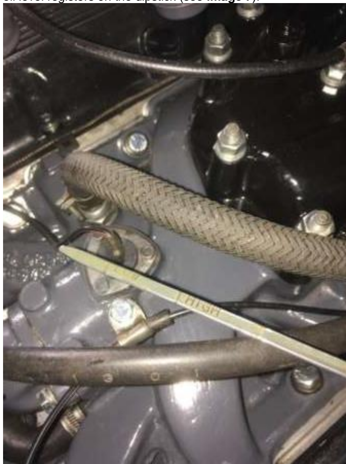
Image 7: Check oil level with the dip stick
