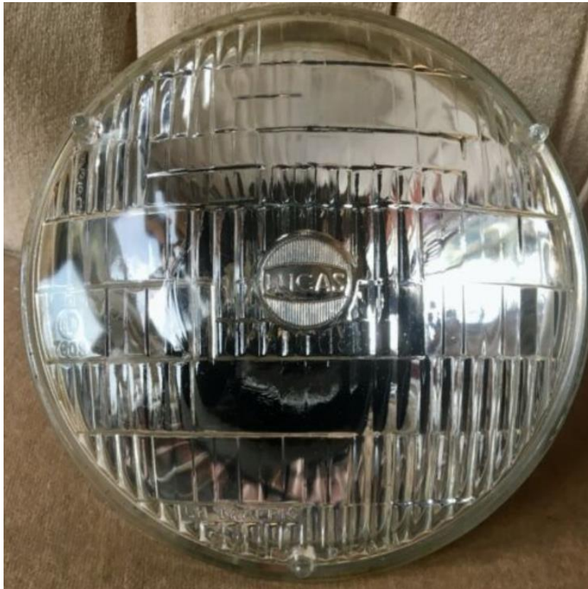
Original headlamp for a chrome bumper MGBGTV8 (RHD) 75W/55W sealed beam headlamp "LUCAS" circular logo in the centre of the domed glass. "LH TRAFFIC" logo in the lower left of the domed glass. No "window" for "pilot" sidelight. Unipart P/N GLU106
