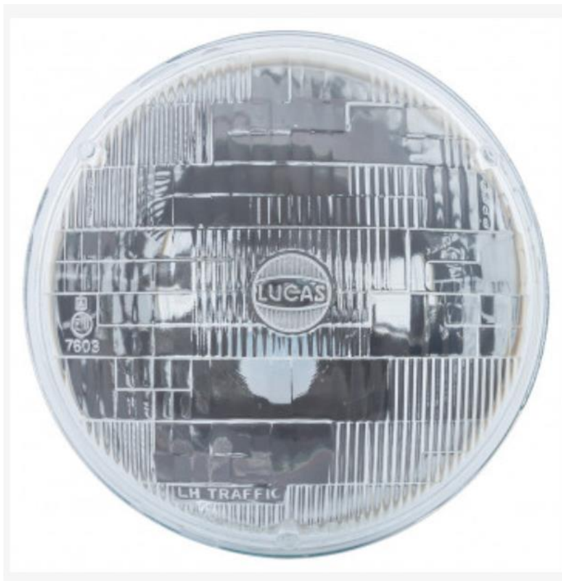
Original headlamp for a rubber bumper MGBGTV8 (RHD) 75W/55W sealed beam headlamp "LUCAS" circular logo in the centre of the domed glass. "LH TRAFFIC" logo in the lower left of the domed glass. "Window" for "pilot" sidelight. Lucas P/N SB7019 Unipart P/N GLU123 , S/S XBC103360
