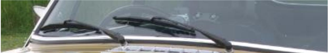
**Pair of Satin Black Bosch SP13 replacement wiper blades**, although not original they are improved they do retain the original Factory spec appearance. Improvements are the quality and performance of the rubber material, a more even pressure on the blade to the screen and improved aerodynamics reducing wind noise.
