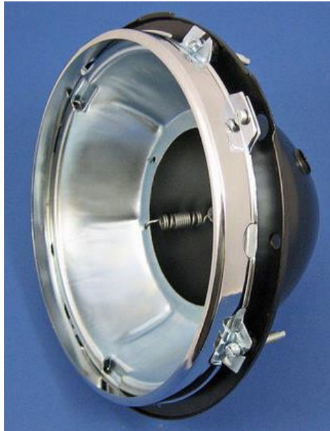
Cibie 7" H4 Halogen headlamp unit with or without sidelight unit (LHD or RHD)
