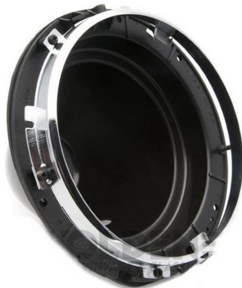
The 2-adjuster backshell. See replacement headlamp unit details.
