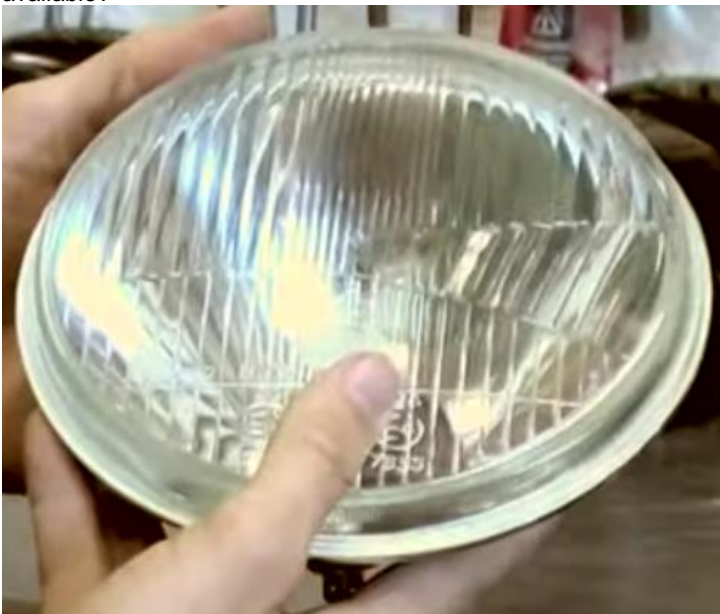
Replacement H4 Halogen headlamp unit with 2-adjuster back shell
