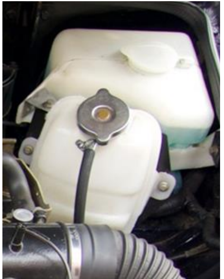
Coolant expansion tank close to the windscreen washer tank.
