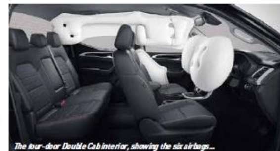
The four-door Double Cab interior, showing the six airbags...
