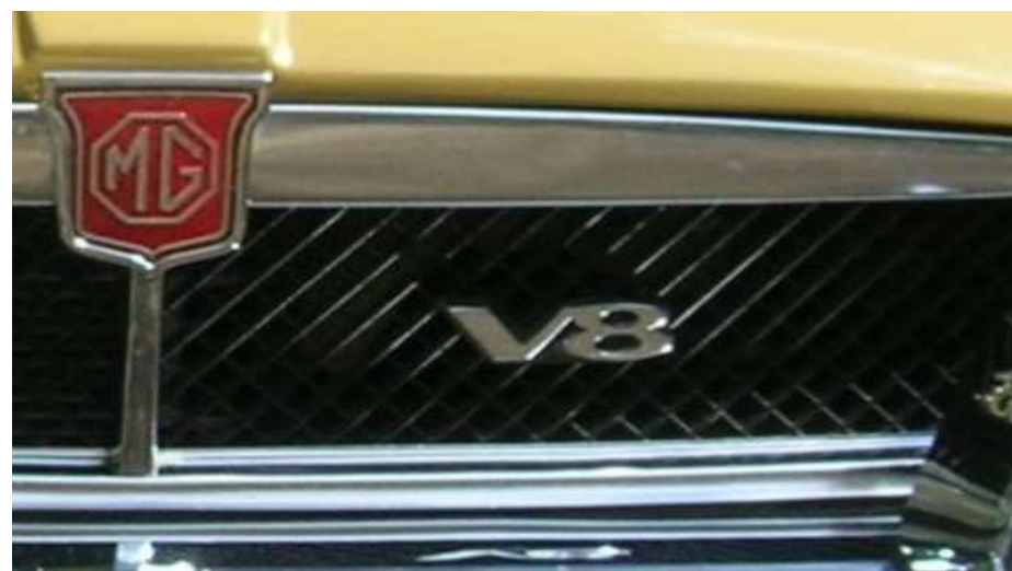
"V8" badge has been fitted to the nearside of the grille but as part of the chrome bumper conversion the restorer has used the wrong grille mesh. The correct mesh has a dominant mesh member going lower left to upper right – see below.
