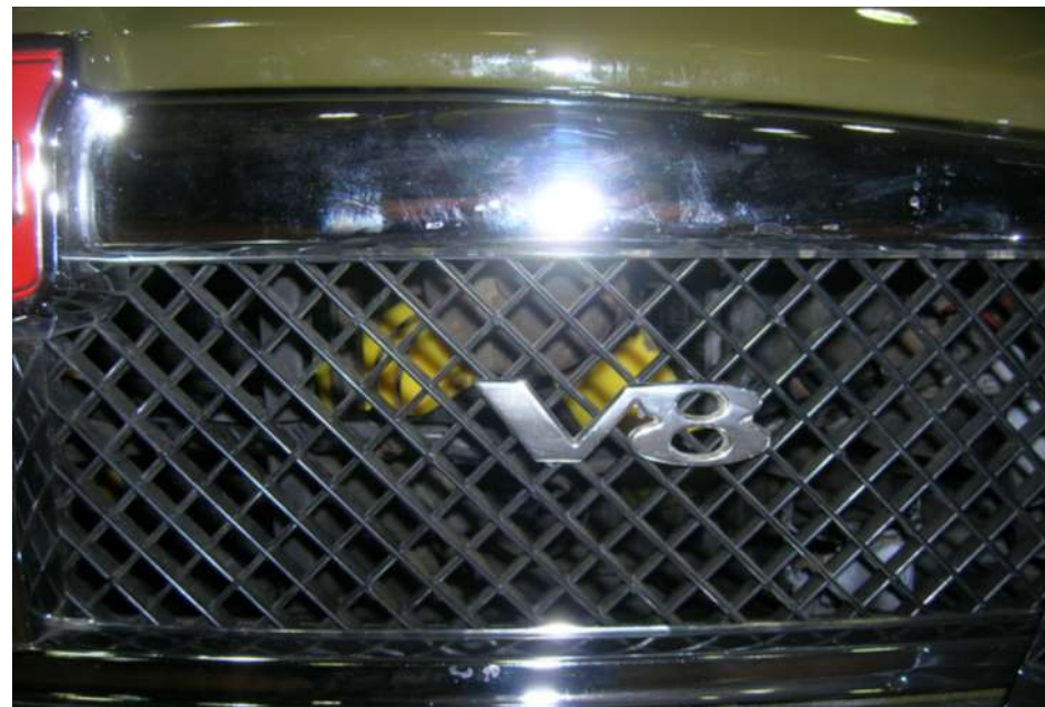
"V8" badge has been fitted to the nearside of the grille but as part of the chrome bumper conversion the restorer has used the wrong grille mesh. The correct mesh has a dominant mesh member going lower left to upper right – see below.
