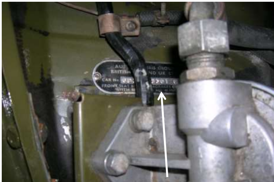
Checking the Car No/VIN on the plate fixed to the offside inner wing adjacent to the remote oil filter shows GD2D1 2301G.
