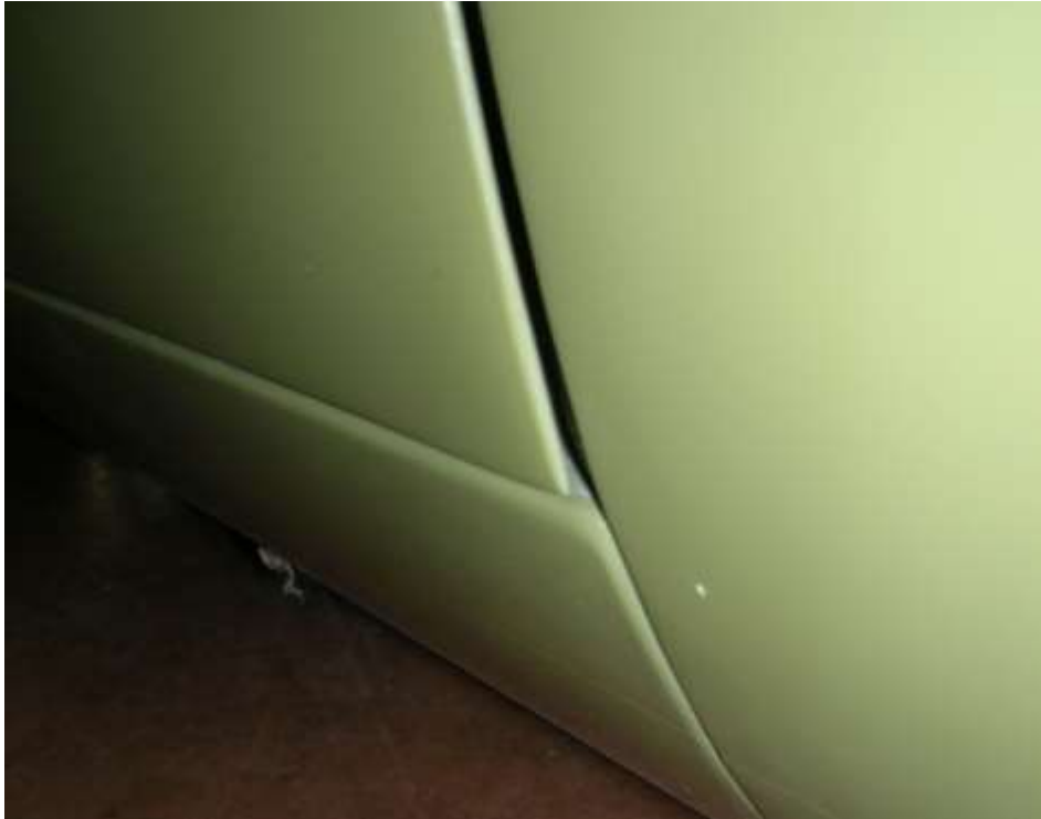
Front edge of the offside door slightly out. The cills looked good.
