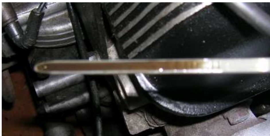
Checking the colour of the engine oil – it was slightly black but reasonably clean. On checking the dampers on the twin HIF SU carburettors, they were very nearly out of oil.
