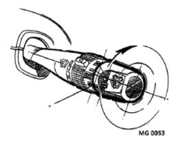
Rotate the switch clockwise to select the wiper speed required;
