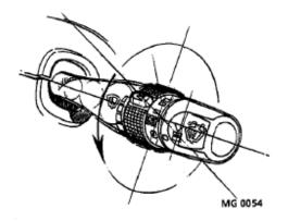
Intermittent Wipe Variable Delay Rotate the switch to vary the delay between wipes.
