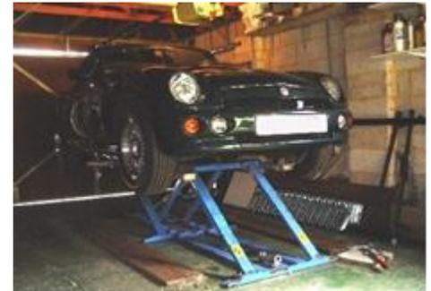
Below: cross member under the RV8 with rubber packing pieces just missing the exhausts – this is Jim's prototype.
