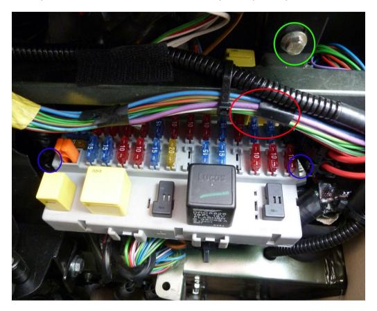
It is possible to replace the relay (circled in red) without removing the fuse board. But this can be fiddly. Alternatively, you can undo the two screws (circled in blue) and pull down the fuse board to gain better access. Note: If you do remove these screws, be careful when replacing the board not to dislodge any of the relays at the top of the board.
