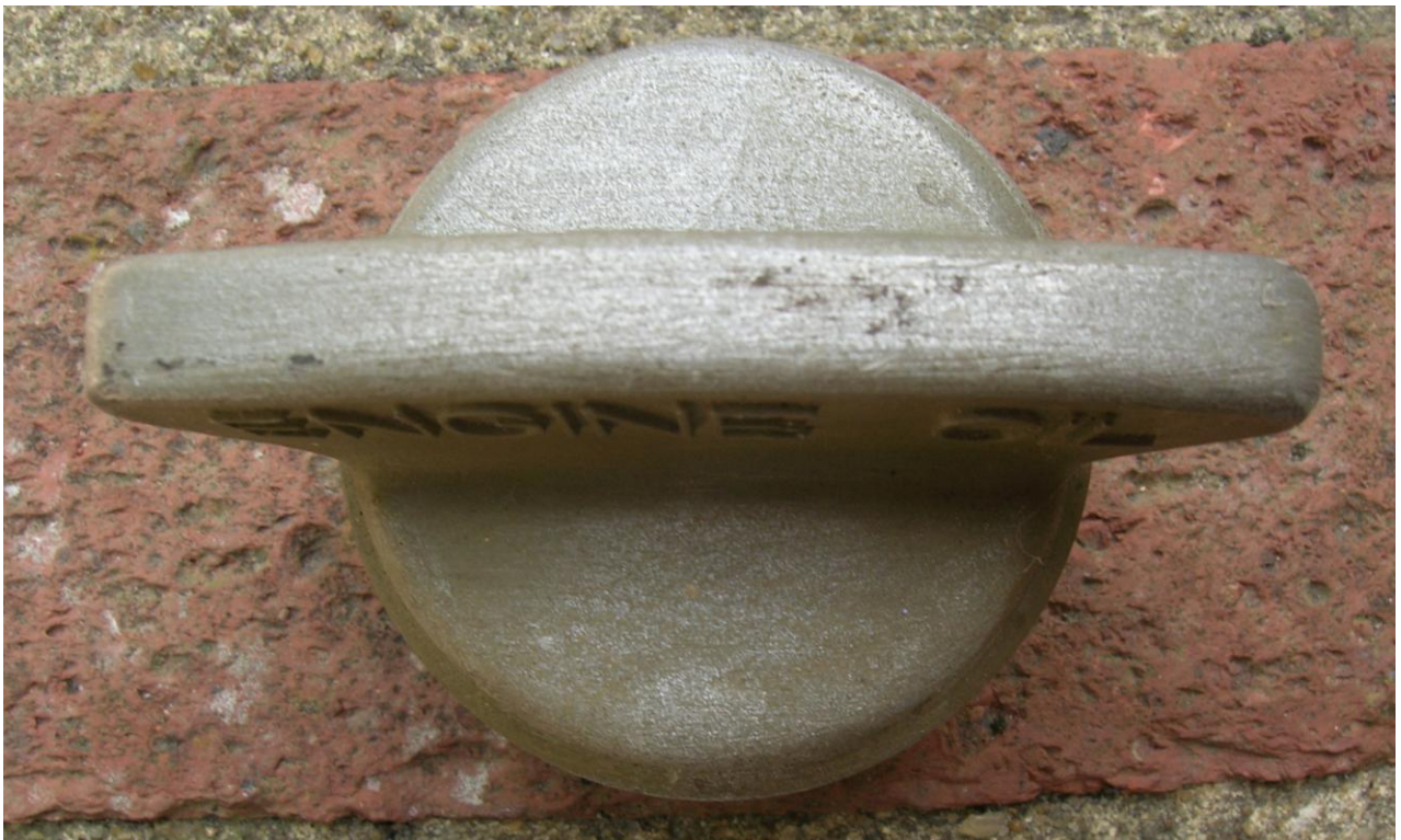
Engine oil cap for an MGBGT V8 rocker cover. Original part number 625038.
