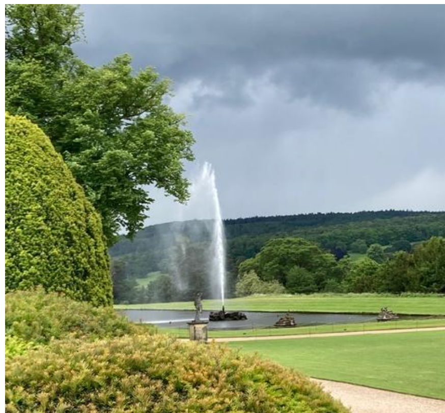
The Emperor Fountain at Chatsworth is on record as having reached the height of 90m (300ft) and powered by the pressure of water dropping 122m, through a 40cm-iron pipe. Link
