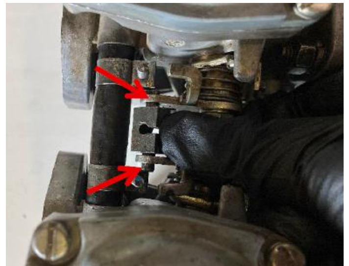
Figure 3 - ears of the hose clip must be oriented away from the choke trunnion
