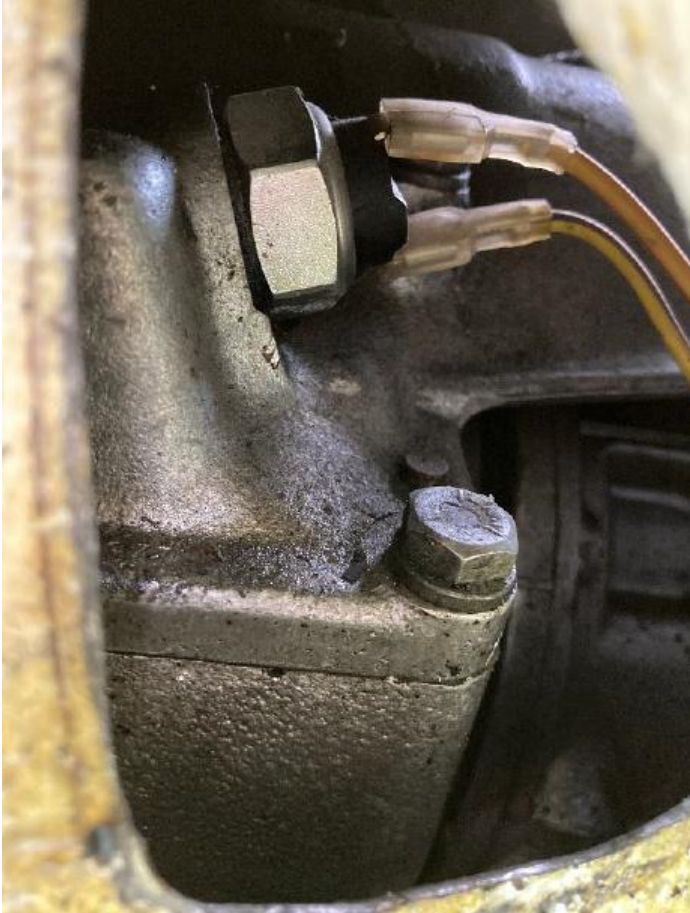
Figure 1 – inhibitor switch accessed by a rubber plug
