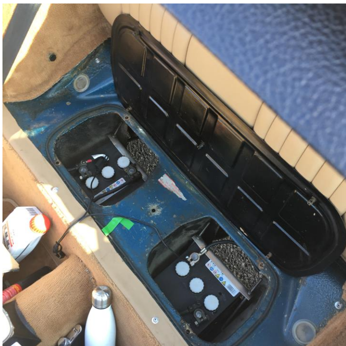
Two new 6-volt batteries firmly strapped in place
