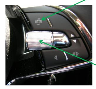
Lane then assist remains off until the engine is stopped and restarted when it will be activated again.
