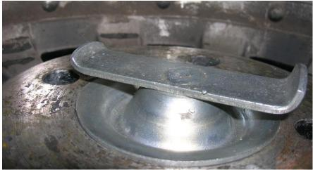
Above: spare wheel holder clamp BHH111 on the inside of the Dunlop composite wheel **on an earlier V8** (VIN 1089). This provides a space to locate a tool box wrapped in a towel.
