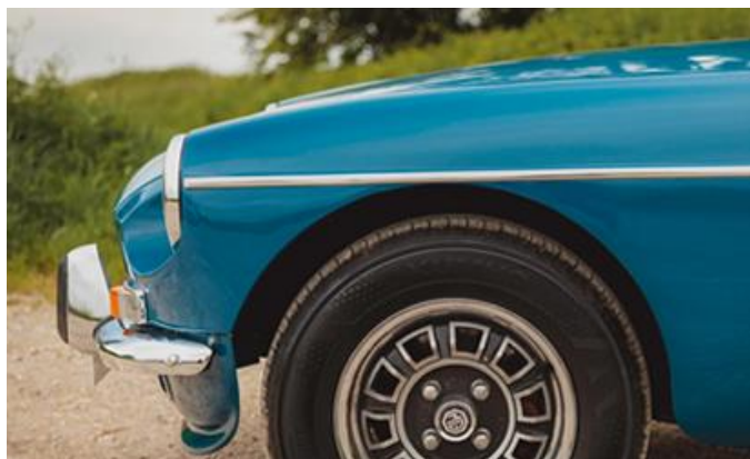
Photos courtesy of Bonhams|Cars Online, showing the Frontline spoiler fitted, replicating the original valance profile
