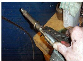
The top bearing is held in place with another circlip. There seems to be two groves each side of the bearing. In the bits I took off, ages ago, there appears to be two circlips, but there is no way this second circlip will fit in the groove as the bearing covers it?
