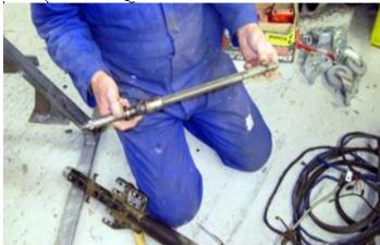
The part I am holding is the inner steering column that I need to repair.
