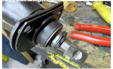
Yes, I did fit the rubber and plate the wrong way round in my excitement of getting the column together at last. This was easily rectified without having to take the column apart again.
