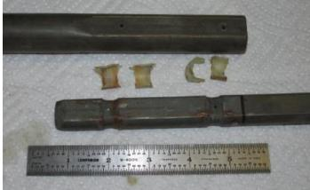
The two parts of the inner collapsible steering that slide inside each other in the event of an accident with the broken bits of plastic that hold the column at the correct length. These I replaced with small screws to hold the two parts together.
