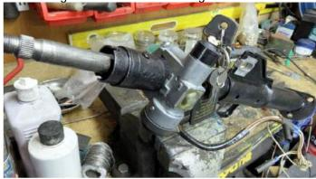
I have not tightened the steering lock fixing bolts to the shear point, just in case I need to take it apart again or the steering lock needs replacing in future.
