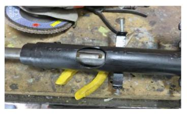
The bearing, spring and circlip at the bottom of the steering column will hold the inner steering column shaft in its correct position.
