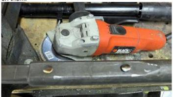
Out came the grinder to grind off most of the head. This does not really matter as I was only using them to hold the inner shaft to the outer shaft. The problem will come if I didn't fix them in the correct place!
