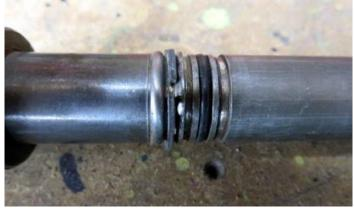
At last, I found out that you do need two circlips to hold the top bearing in place. The standard bearing that BL used was also not the correct size for the steering column shaft. You can see in this photo the 'O'-ring that they added to the shaft to stop the inner race of the ball race rotating on the shaft. Another BL bodge!
