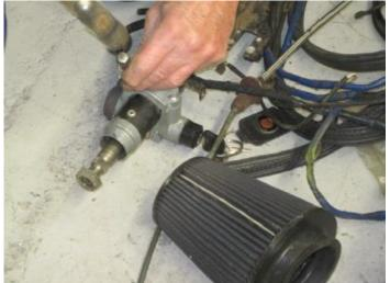
The bolts for the steering column lock are 'shear bolts'. When the steering column was fitted in the Factory, the spanner part of the bolt shears off, leaving no means to remove them. This is to slow down thieves. If you centre
