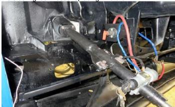
It was easier fitting the steering column to the body with the shell upside down on the spit".
