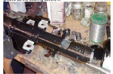
Over the bearing sits a rubber collar to take up the space, and make the bearing fit in the outer column. It looks like a bit of a British Leyland bodge to me, but I
