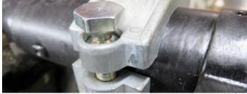
The next job was to bolt the steering lock back onto the other steering column. This photo shows clearly the 'shear bolt' holding the lock onto the steering column.
