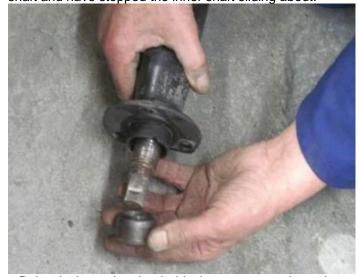
Below is the spring that holds the centre steering column in place. The circlip at the bottom looks as if I need to replace it. As it is not available from MG suppliers I will
