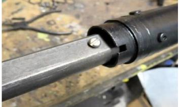
The inner shaft would not slide down the outer steering column. The M4 screws I had used had too larger heads on them.
