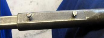
Unfortunately, I forgot to take photos before I repaired this part. Normally, there are some pins where I have installed the 4mm screws. They fit into some plastic inserts in the bit underneath the screws you can see in the photo. What I have done is tap the holes where the pins fitted and replaced them with screws. The column should then still collapse in an accident. The screws just press on the inner shaft and have stopped the inner shaft sliding about.
