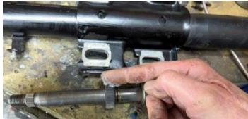
I wiped the bearing cover with Vaseline to help the bearing and its cover (spacer) to slide into its correct place inside the outer column.
