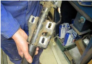
This photo shows the crumple zone part of the steering column where my right hand is holding the column. The three aluminium 'bits' are the top bolts mountings for attaching the steering column to the bodyshell by the dashboard.
