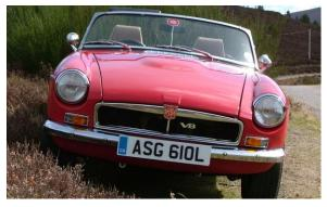
The V8 Roadster built by Geoff King was the inspiration for my MGBGTV8 conversion. Both conversions have the Hoyle front and rear IRS upgrades which transform the handling of the car.
