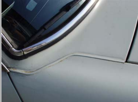
Rust emerging on the front wing dog-leg seam
