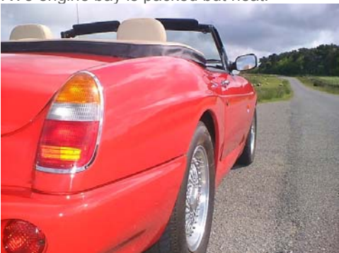
The cleverly fashioned bumpers in the body colour suit the flowing lines of the car – note the rear light cluster, another item that was different to the part on the earlier V8 model. (Photo: Flame 2195, Bill Wood)
