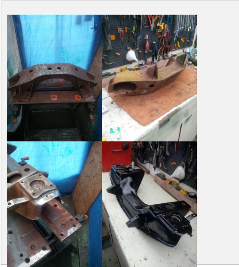
The next job was to renovate the wishbone pivots which are re used with the evolution 3 system and prepare all of the other components ready for installing on the cross member. This involved cleaning, de rusting, de greasing and painting all the various parts.
