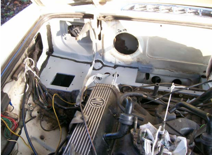
Heater matrix removed and offside portion of the bulkhead shelf cleaned up and undercoated. (Photo: Clive Wagerfield)
