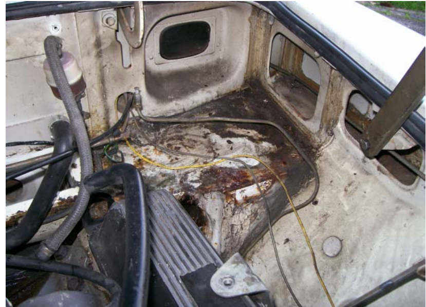
Nearside portion of the bulkhead shelf where corrosion under the servo unit is seen. Below, the area cleaned up and undercoated. (Photo: Clive Wagerfield)
