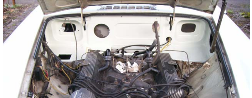
Completed refurbishment of the bulkhead shelf ready for reassembly of the brake and clutch master cylinders, heater matrix, brake servo and screen washer bottle. (Photo: Clive Wagerfield)
