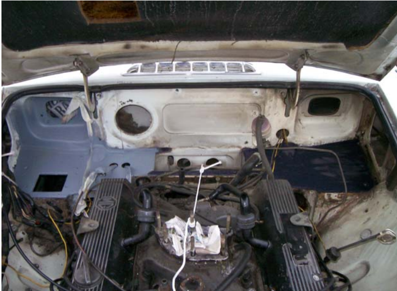
Heater matrix removed and offside portion of the bulkhead shelf cleaned up and undercoated. (Photo: Clive Wagerfield)
