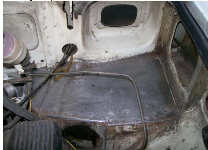
Nearside portion of the bulkhead shelf where corrosion under the servo unit is seen. Below, the area cleaned up and undercoated. (Photo: Clive Wagerfield)
