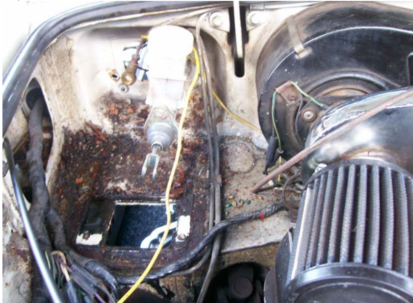
Offside portion of the bulkhead shelf where corrosion in the pedal box area is seen on so many cars. (Photo: Clive Wagerfield)
