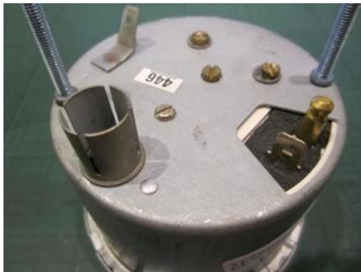
Rear view of the unit, showing the blade terminals for the power supply and earth, together with the "bullet" terminal which is connected to the coil and picks up the pulses.
