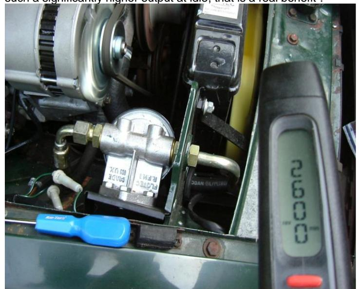
Upgraded alternator with the cooling fans at 2,600rpm.
