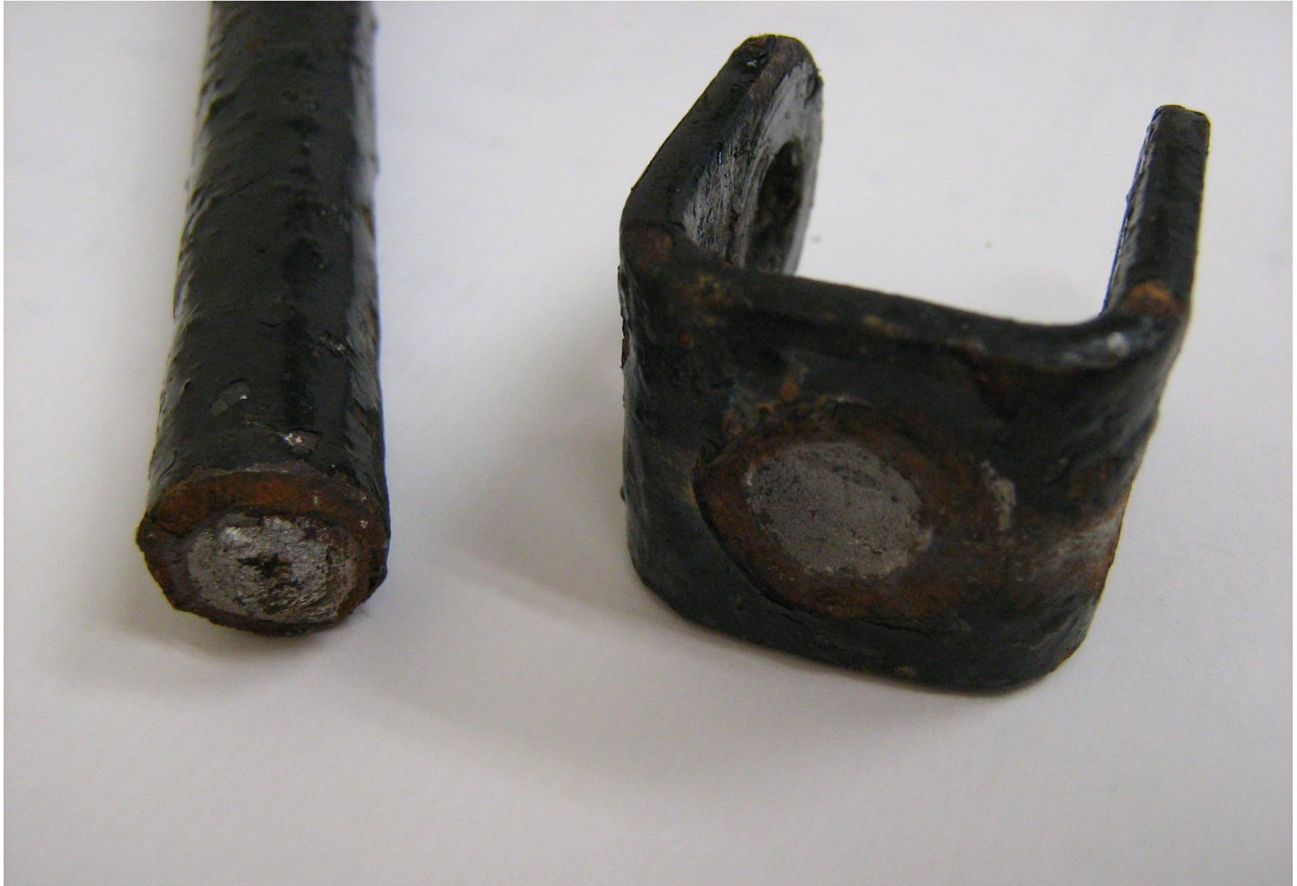
Broken drop link (anti-roll bar link) on an MGBGTV8
