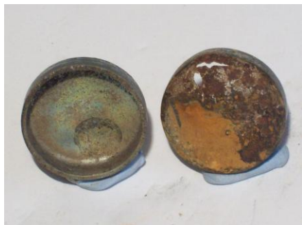
Core plug appearance. LH plug in good condition. RH plug seen from wet side and corroded right through.
