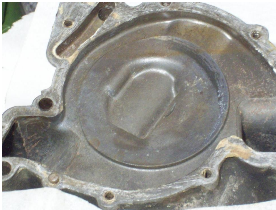
Front cover showing excellent condition after 160,000 miles on correct coolant treatment and maintenance
