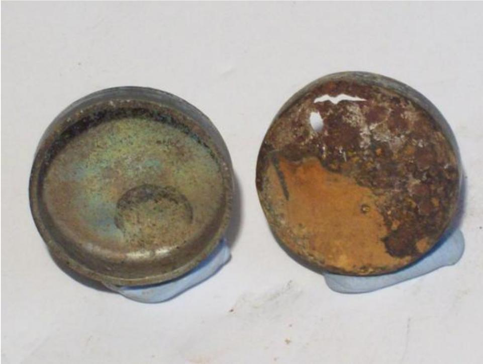
Core plug appearance - LH plug is in good condition but the RH plug seen from wet side is corroded right through.
