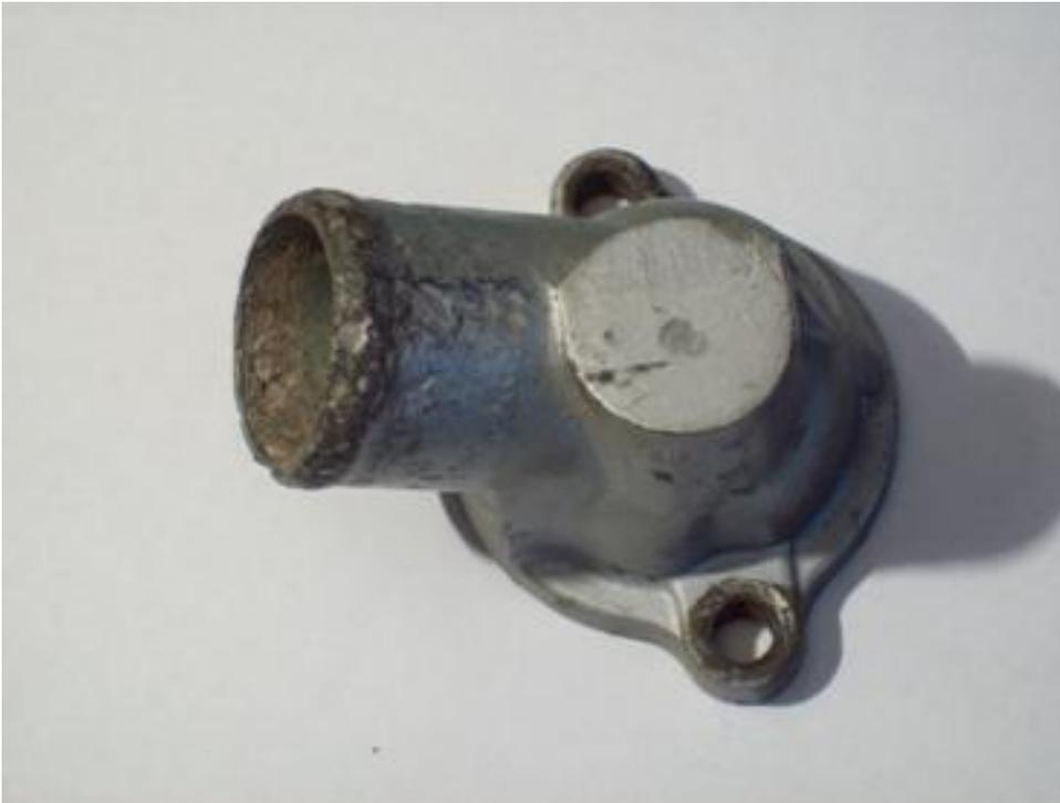
Thermostat housing from a Rover V8, the elbow is at a different angle than the MG V8 uses. Unknown age or coolant treatment; but heavy corrosion in the hose bead/sealing area and some very deep pits inside the casting. It is unreasonable to expect any hose/clip combination to seal for long without leaking. Replace components in this condition.
