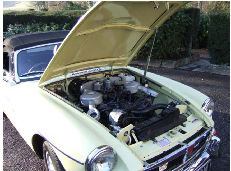
Engine installation uses the original Factory layout with twin SU carburetors and air cleaners. (Photos: Roy Crosland)
